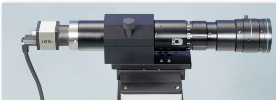
high-performance 10-fold zoom lens with software-controlled optic alignment for adjusting the observation angle and for autofocus
