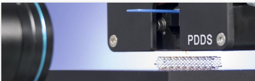
measurement on a coronary stent with the picolitre dosing system PDDS
