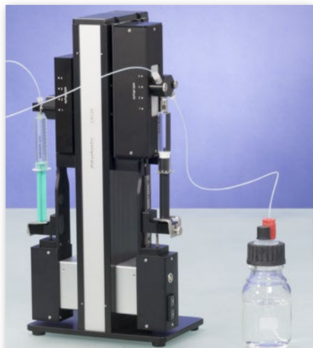
liquid dosing unit LDU 25
