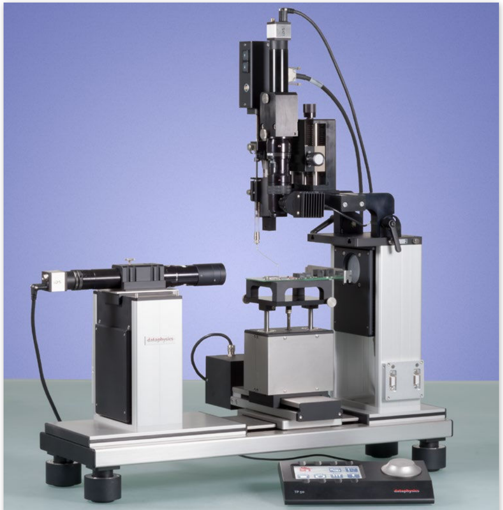
Topview Video System with collimated coaxial illumination TVS-C on an OCA 100
