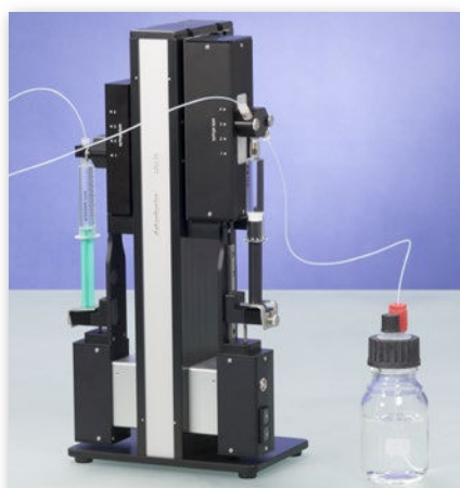
Fig. 5: The LDU 25 liquid dosing unit allows operators to change the concentration inside the solution automatically.
