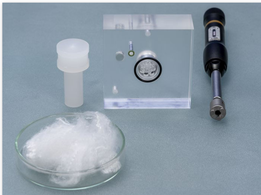
Fig. 4: MC-ZPA/PF measuring cell for fibres, powders, and granulate material together with sample preparation tools
